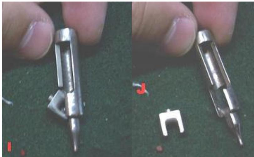
When reinserting the "Striker Spacer" (#21) it does not matter which side goes in first, both are the same.
