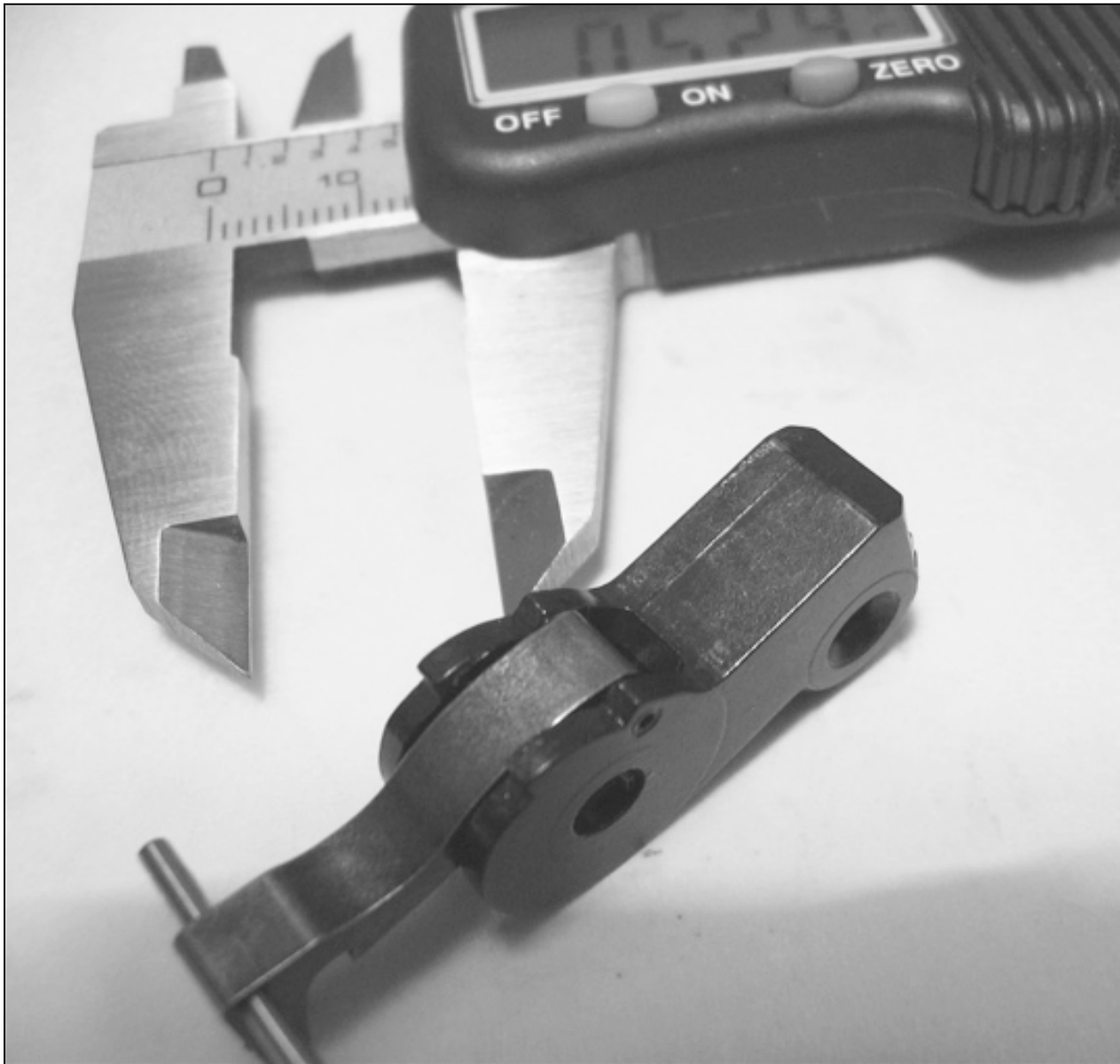
New style hammer ready for re-profiling.
