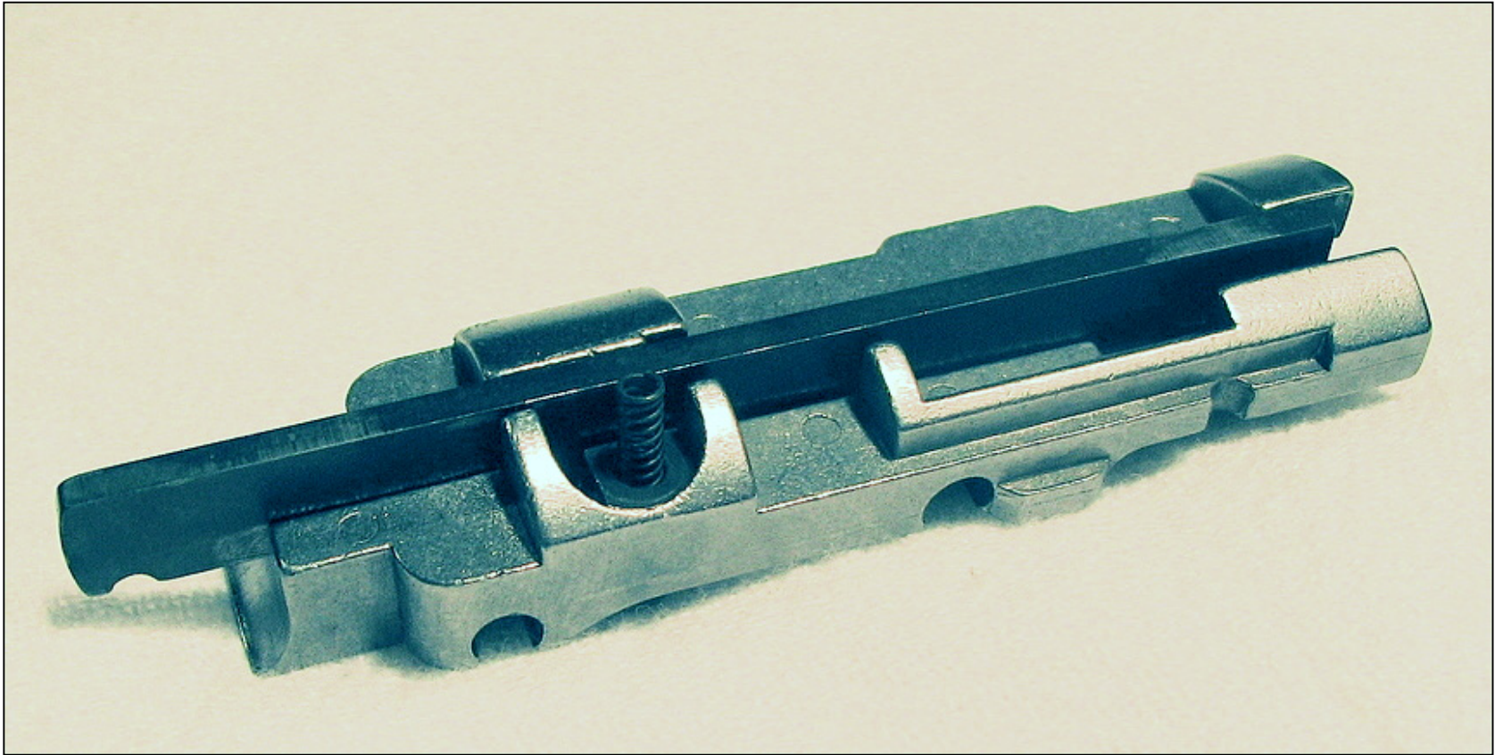
This photo shows the properly reassembled breech block.
