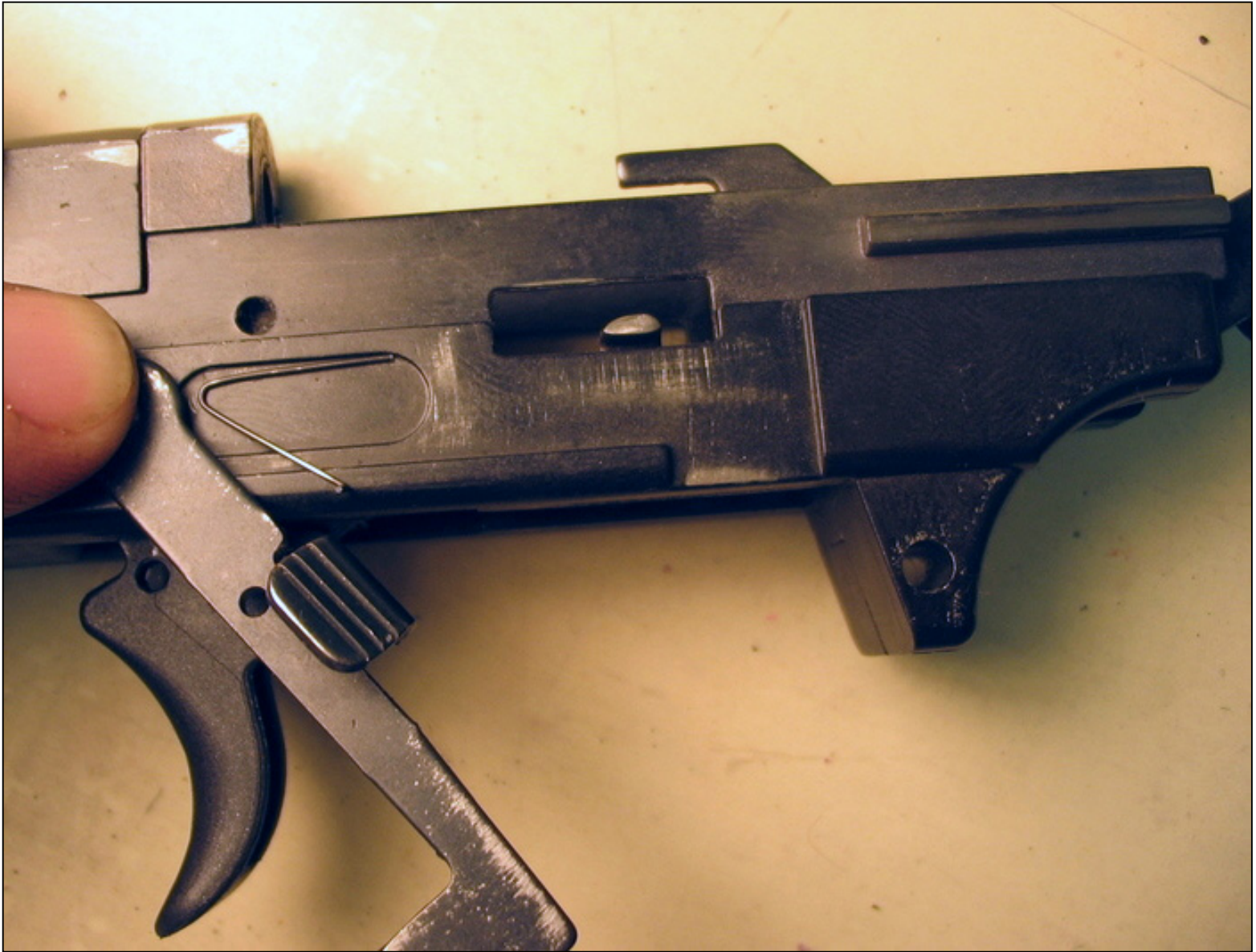
Photo of the proper position of components upon reassembly of the slide stop mechanism.
