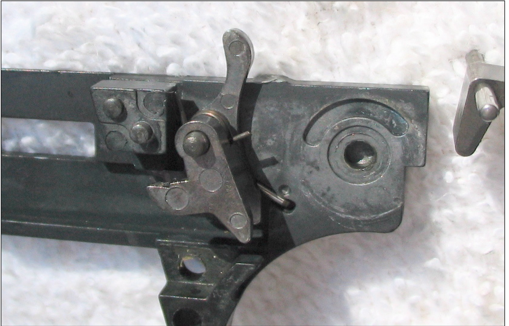
Sear, notice spring position. The ear sticking up will rotate forward to a horizontal position upon reassembly and will have to be pressed down for reassembly of the hammer assy.
