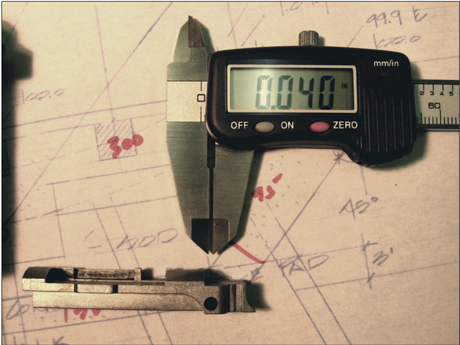
There is 0.040 inch of metal between the bottom of the breech block retaining pin hole and bottom of the breech or just enough to remove 0.020 so the hammer tip will no longer drag.
