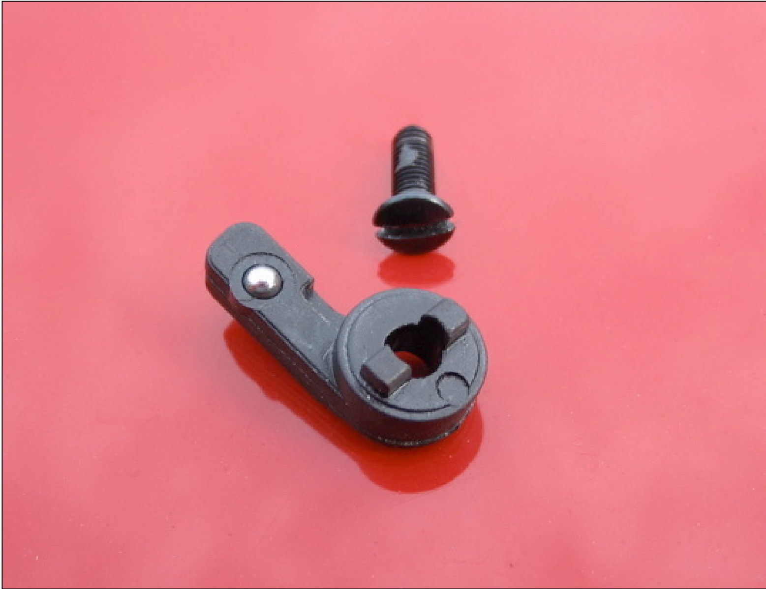
Picture of the safety lever and associated screw.
