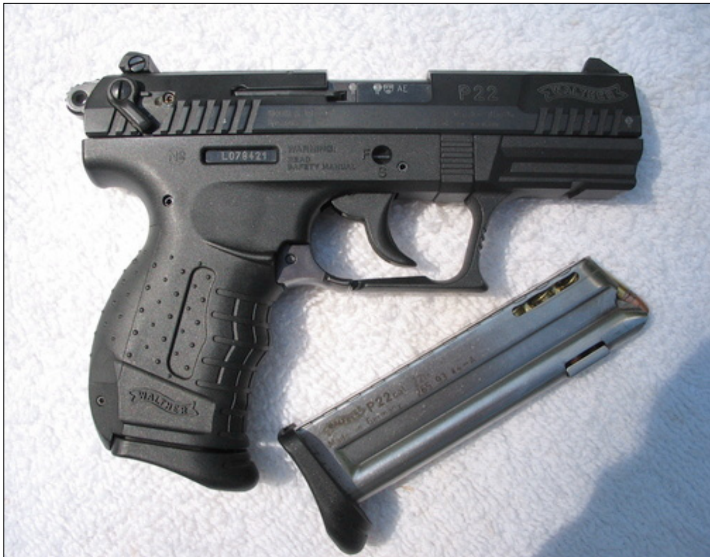
The P-22 ready for disassembly, safety on, the short barrel model without the barrel stabilizer. With exception of removal/reassembly of the stabilizer, both pistols 5" or 3.4" are the same.
