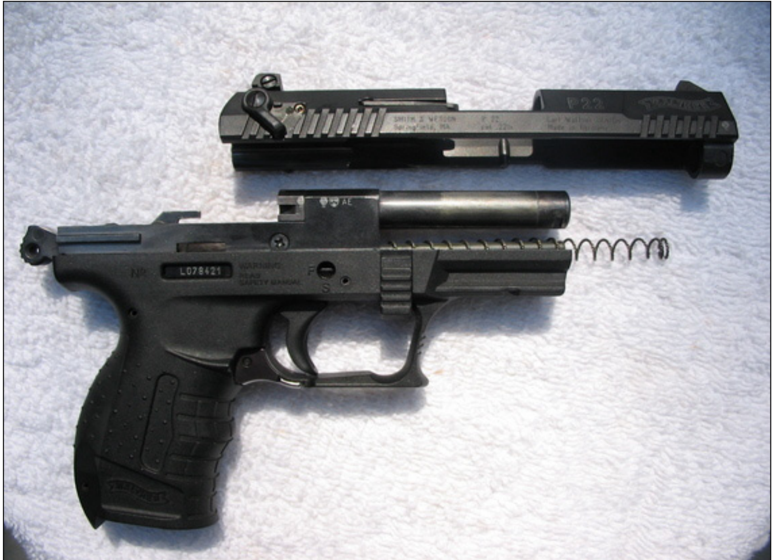
This photo shows the slide off while the slide spring and guide bar are still in place. The same position they will have upon reassembly.
